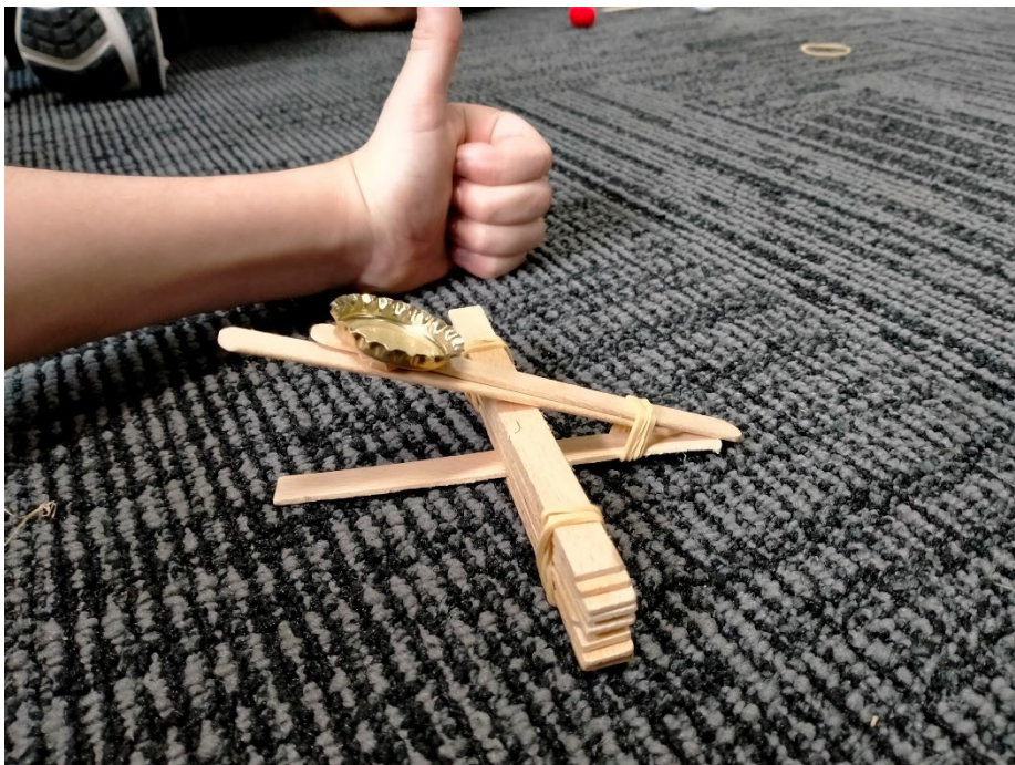
Figure 1 (b) An early modification to increase potential elastic energy to the lever – extended lever modification
