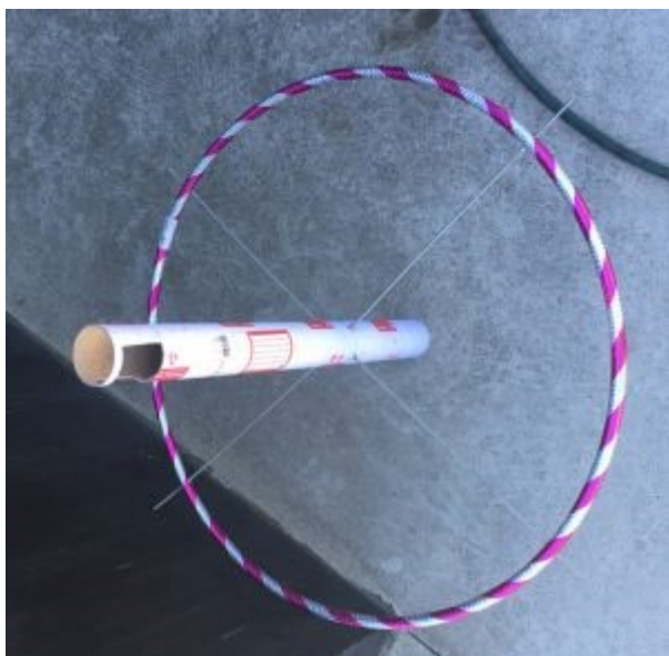
Figure 3. The finished Maunder and Hunt's Very Famous Rainbow Finder. Note the viewing window cut into the end of the tube.
