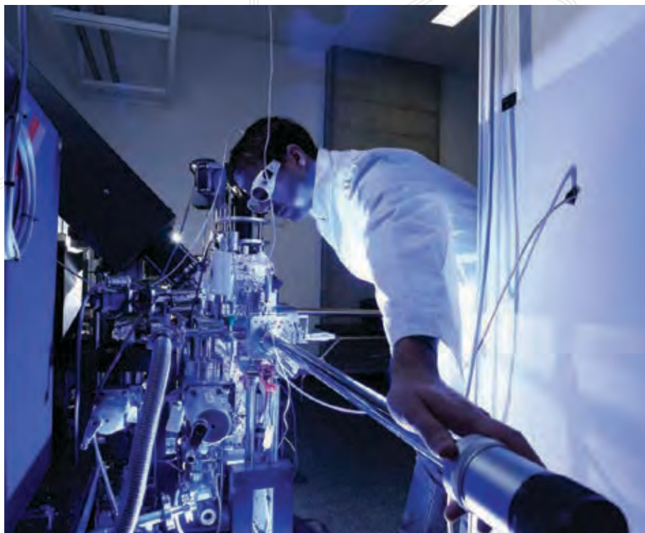
Research fellow Daniel Sando with oxide pulsed laser deposition (PLD) chamber used to fabricate thin-film samples with very high crystalline perfection, preparing interfaces required for FLEET Research theme 1
